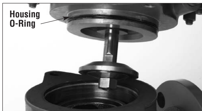
Fig. 42 Installing the Actuator on the Body.
