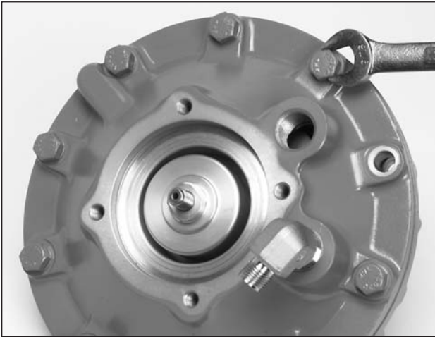
Fig. 29 Removing the Housing Cap Screws.
