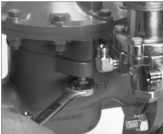
Fig. 17 Tightening the Body Cap Screws.
