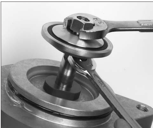
Fig. 13 Hold the Stem while tightening the Stem Nut.
