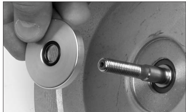
Fig. 32 Installing Lower Diaphragm Retainer.
