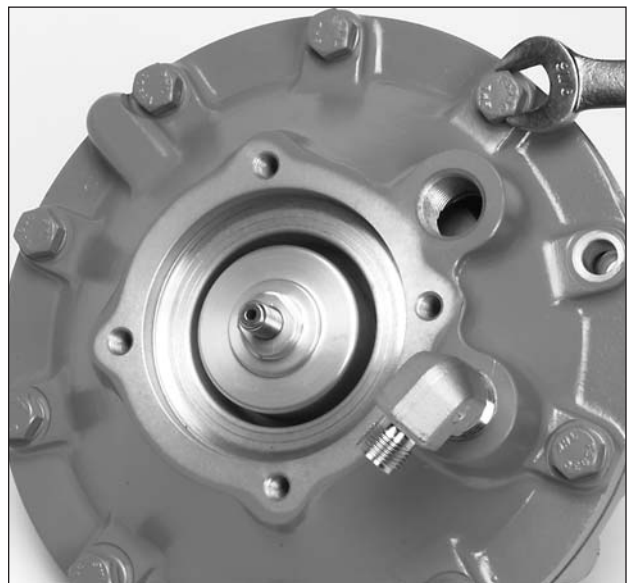
Fig. 35 Install the remaining actuator Cap Screws.
