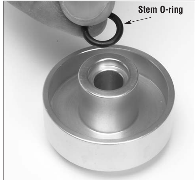
Fig. 31 Inspecting Stem O-ring.
