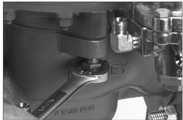
Fig. 43 Tightening the Body Cap Screws
