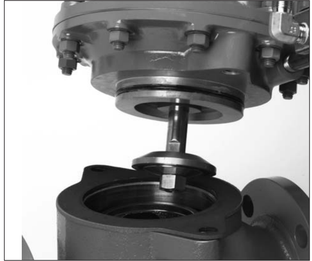
Fig. 6 Remove Actuator from Regulator Body.
