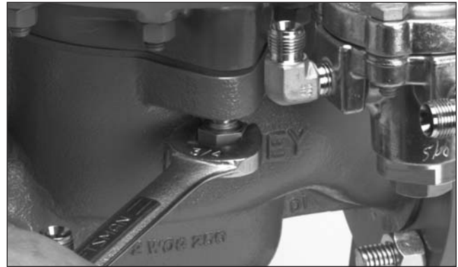
Fig. 27 Tightening the Body Cap Screws.
