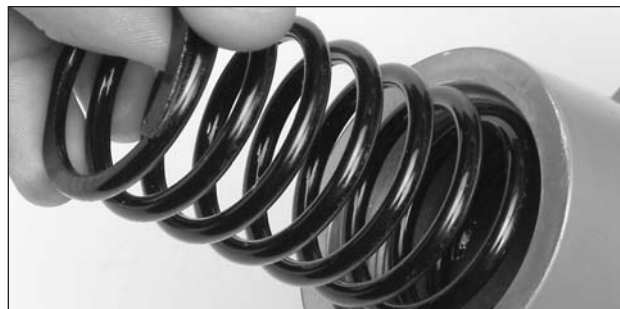
Fig. 41 Installing the Main Spring
