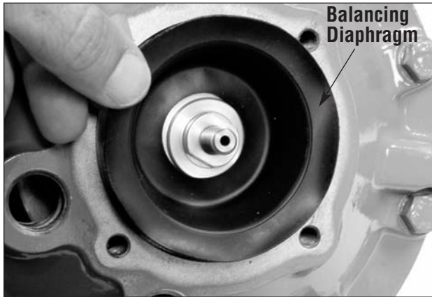
Fig. 36 Replacing the Balancing Diaphragm
