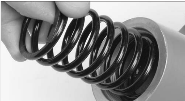
Fig. 25 Installing the Main Spring
